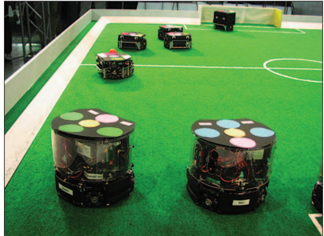
Figure 7. RoboCup competition with soccer game field. The robots work together in both defensive and offensive plays against the opposing team. Each robot has its own controller. A vision system is required to track the locations and actions of all robots and the ball on the playing field. A centralized controller uses this information to send play information to the individual robots so they can work together against the opposing team.
